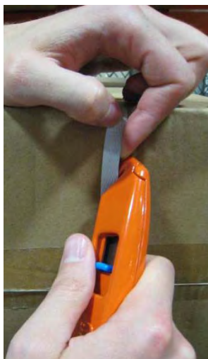
Hook the strap with the beak of the knife without extending the blade.
